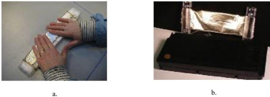
Figure 1. (a) A rolled multilayer DEAP composite pressed to form a flat structure. (b) A photograph of the final assembly of Poly Power flat DEAP actuator (Rahimullah Sarban, 2011)
