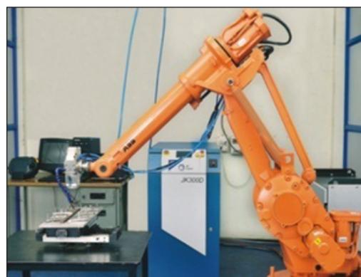
Figure 3. Experimental set-up for pulsed LBW of Ti-6Al-4V alloy
